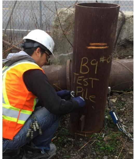
Figure 6: EXP Services performing a PDA Test on the impact of the EML30 Drop Hammer
