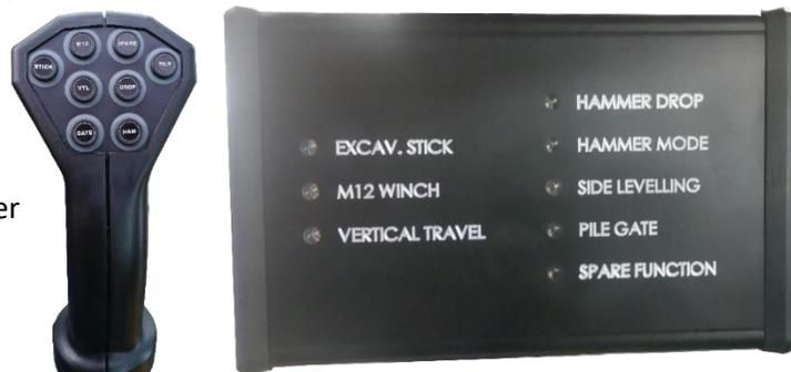
Figure 5: Cab Control Joystick and Mode Panel
