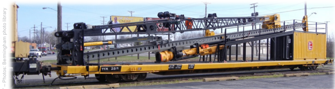
Berminghammer L-15 Vertical Travel Leads, and B-21 Diesel Impact Pile Hammer on a lead car
