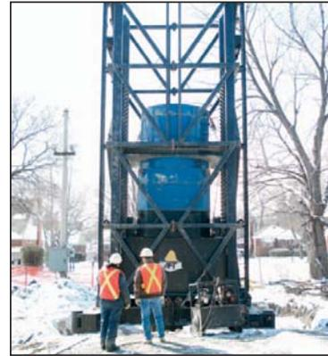
The third pile that was tested showed results similar to that of the first pile. A similar attempt to improve the pile capacity through cyclic loading (4-cycles, see below) showed no improvement in the pile capacity. This testing proved without a doubt that the bearing layer (a dense sand) was not capable of supporting the required ultimate capacity of 10,000-kN. Additional "remedial" foundations were required to supplement these foundations -- proof that load testing is a good idea!
