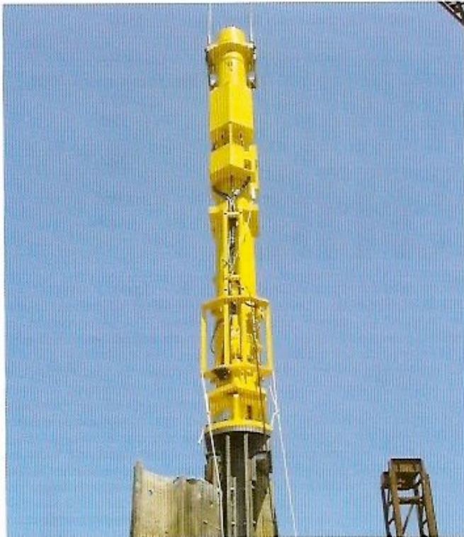
Modern diesel hammers have addressed controllability and environmental issues and have high efficiency and low cost.
