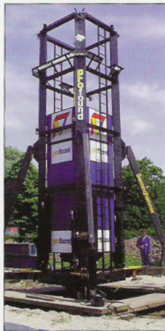
LEFT: A recent development of the technique uses water as the reaction mass when testing on or near water. RIGHT AND ABOVE: The test uses a reaction mass launched by generating high pressures in a pneumatic cylinder by burning a special fuel.
